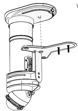
**F.** The mark on the tube must be at or below the waterline.
