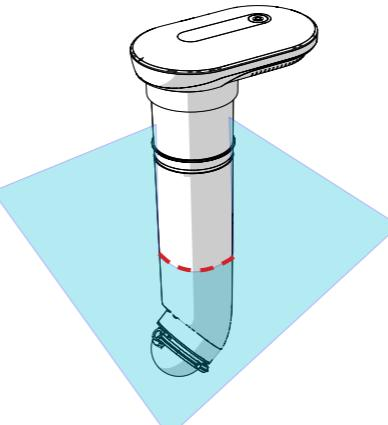
**G.** Insert the pool unit pin in a straight or a rotated docking position and connect to power.
